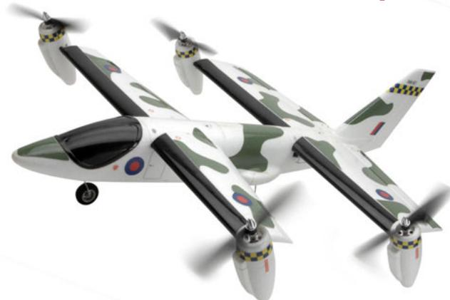
The Ripmax Transition is a VTOL aircraft rather than a pure helicopter. In hover mode it flies much like a quad copter, but as the press of a button the motor pods and rotors swivel forward. It then becomes a conventional aircraft, using its wings for lift. The Transition comes without a transmitter and receiver and but can be flown on any 5 channel or higher set.
