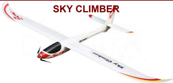
The Sky Climber is a 2m span electric glider made from tough EPO foam. It has a powerful brushless motor and a folding prop and features four channel control including ailerons so is quite manoeuvrable yet not too difficult to fly.
