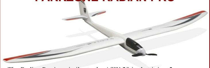
The Radian Pro is similar to the ASW 28 in that it is a 2m span electric glider made from tough EP foam. The main difference is that the Radian Pro has flaps which can be used to increase lift at low speeds and to slow the model down for landing. The motor is used to climb and is then switched off and the aircraft then becomes a glider. Running time of the battery is around 10 minutes, but much longer flights can be had if there is good thermal lift around.
