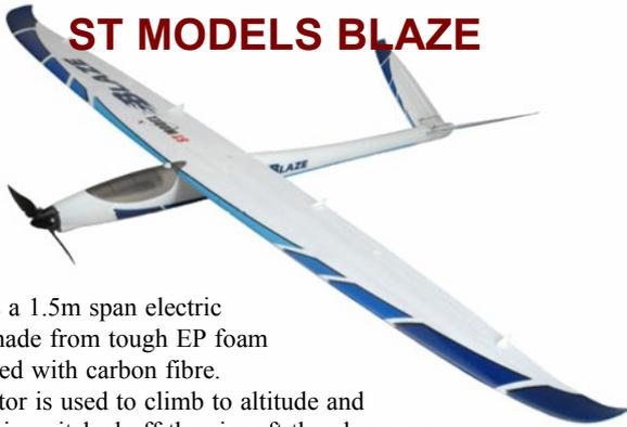
The ST Models Blaze is a 1.5m span electric glider made from tough EP foam reinforced with carbon fibre.
