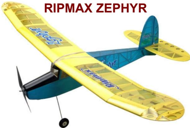
The airframe comes built and covered and just some final assembly to fit the R/C is needed to get it flying.
