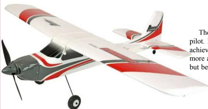
The Gamma Pro is a trainer that can be programmed to suit the ability of the pilot. In beginner mode it will restrict the maximum bank angle that can be achieved and will return the aircraft to level flight if the controls are centred. In more advanced modes the limits are relaxed to allow manoeuvres to be performed but beginner mode can be reinstated at the flick of a switch.
